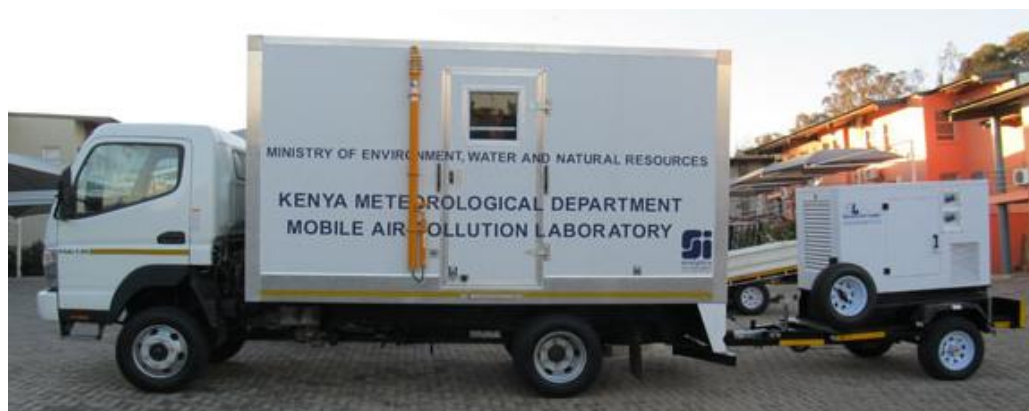
Fig. 1. Mobile Air Pollution Monitoring Laboratory used in this study
