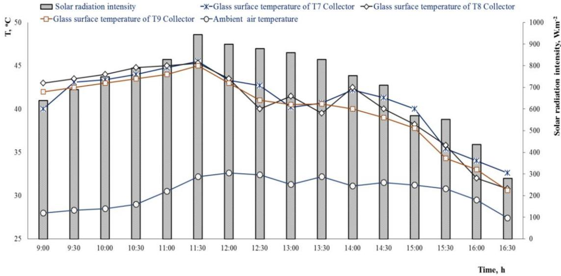
**Fig. 10. The effect of installation height of the collectors to glass surface temperature during the daytime.**
