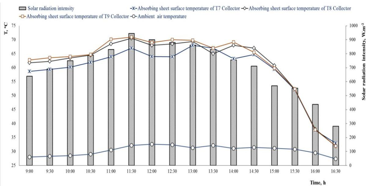
**Fig. 11. The effect of installation height of the collectors to absorbent plate temperature during the daytime**
