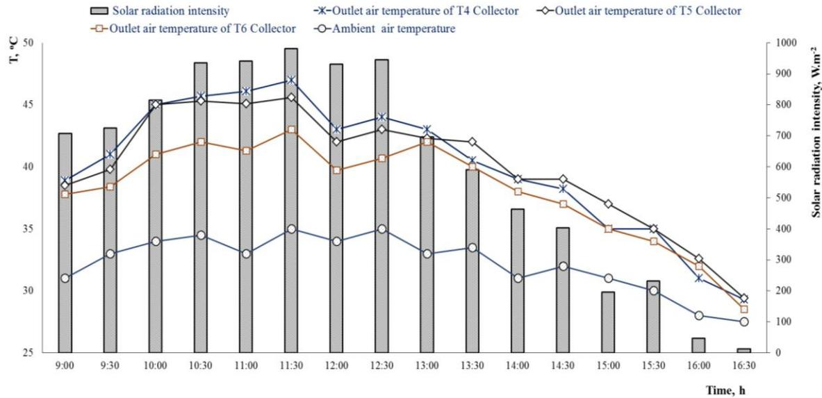
Fig. 6. The effect of absorbent material of the collectors to outlet air temperature during the daytime.
