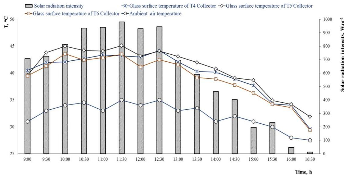
Fig. 7. The effect of absorbent material of the collectors to glass surface temperature during the daytime.
