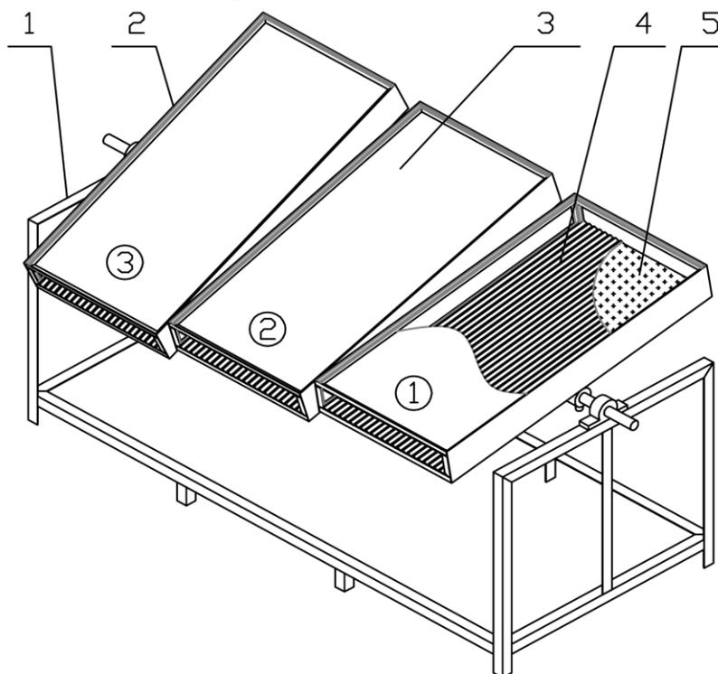
Fig. 1. Experimental system: 1. Main frame; 2. Collector frame; 3. Glass cover; 4. Absorbent plate; 5. Insulation sheet.
