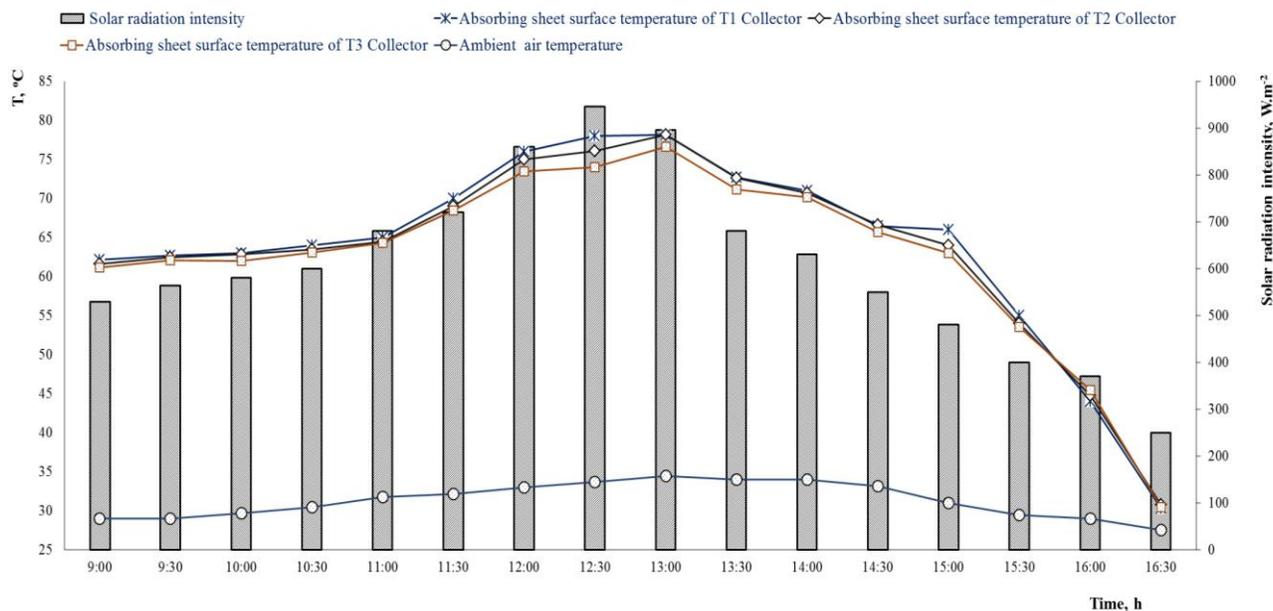
**Fig. 5.** The effects of the tilt angle of collectors to absorbent plate surface temperature during the daytime
