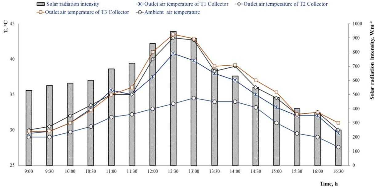
**Fig. 3.** The effects of the tilt angle of collectors to outlet air temperature during the daytime.
