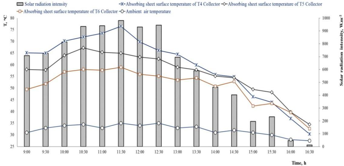
**Fig. 8.** The effect of absorbent material of the collectors to absorbent surface temperature during the daytime.
