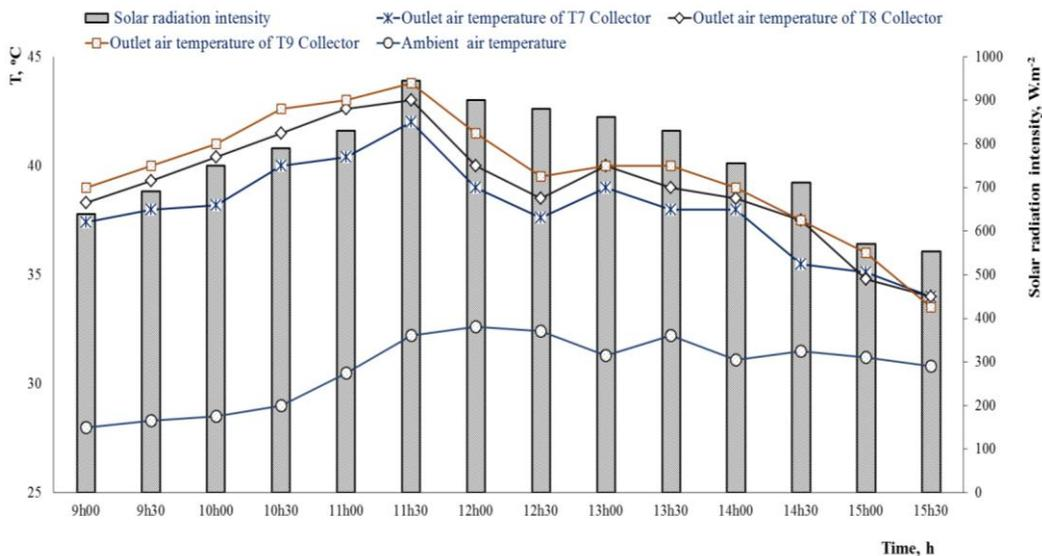
**Fig. 9.** Effect of installation height of the collectors to outlet air temperature during the daytime.
