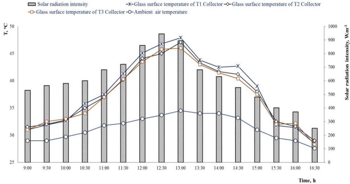
**Fig. 4.** The effects of the tilt angle of collectors to glass surface temperature during the daytime
