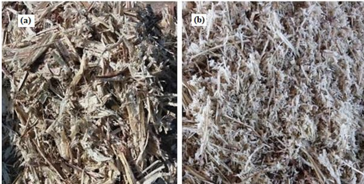
Fig. 7. Comparison of Bagasse Shape Obtained from (a) Conventional cane crusher (b) Modified cane crusher
