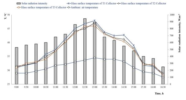
Fig. 4. The effects of the tilt angle of collectors to glass surface temperature during the daytime
