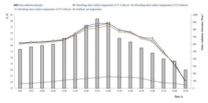
Fig. 5. The effects of the tilt angle of collectors to absorbent plate surface temperature during the daytime
