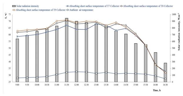
Fig. 11. The effect of installation height of the collectors to absorbent plate temperature during the daytime
