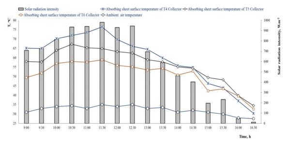
Fig. 8. The effect of absorbent material of the collectors to absorbent surface temperature during the daytime.
