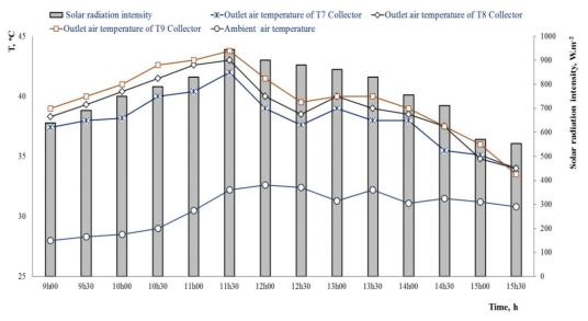
Fig. 9. Effect of installation height of the collectors to outlet air temperature during the daytime.
